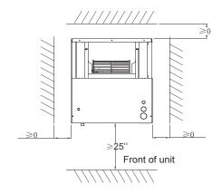
Fig.3 CLEARANCES IN THE VERTICAL POSITION
