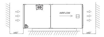
Fig.2 CLEARANCES IN THE HORIZONTAL POSITION
