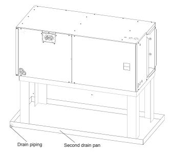
Fig.5 INSTALLED HORIZONTALLY
