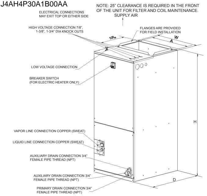
UPFLOW UNIT SHOWN; UNIT MAY BE INSTALLED UPFLOW, DOWNFLOW, HORIZONTAL RIGHT, OR LEFT AIR SUPPLY.
