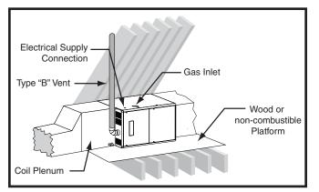
Figure 7. J801X\*U Horizontal Installed on a Platform
