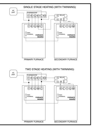
Figure 18. Emerson Single & Two Stage Twinning
