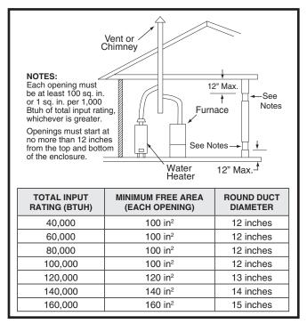
Figure 2. Combustion Air Drawn from Inside
