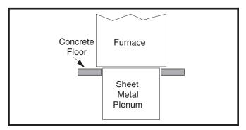
Figure 9. Furnace on a Concrete Slab
