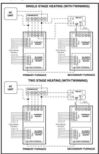
Figure 17. Single Stage Twinning
