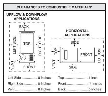
$^{\dagger}\text{Allow}\,24$  in. minimum clearance for servicing. Recommended clearance is 36 in.
