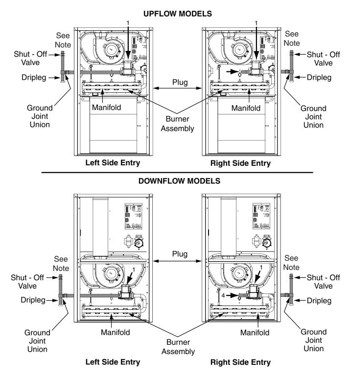
**NOTE:** Some utilities require Shut- Off Valve to be 4 - 5 feet above floor. **Figure 13. Typical Gas Connections**
