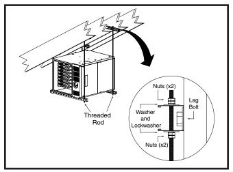
Figure 8. J801X\*U Horizontally Suspended in Attic
