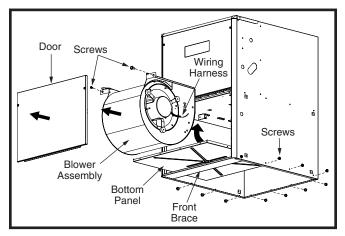
Figure 11. Bottom Panel Removal
