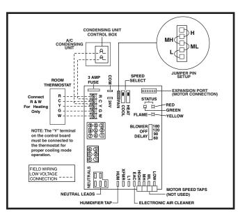
Figure 15. Nordyne/UTEC Low Voltage Field, Fourwire Heating/Cooling Applications
