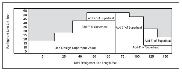
Use the final superheat value, refrigerant temperature and pressure from STEP 4, to determine the proper suction gauge pressure using Table 14-1.
